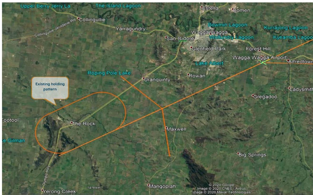
**Figure 1:** Existing approach procedure to RWY 05 and existing holding pattern (orange)
