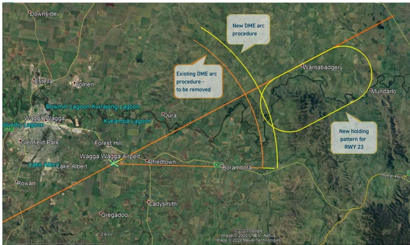
**Figure 2:** Existing ILS/LOC approaches and DME arc (orange) for RWY 23 and new DME arc and holding pattern (yellow)
