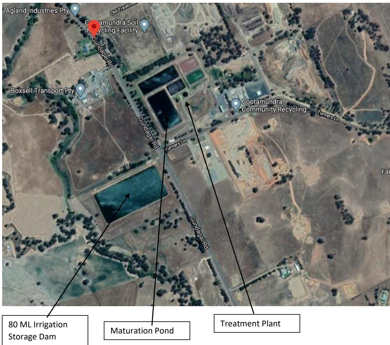
Figure 1- Layout of Cootamundra Sewage Treatment Plant
