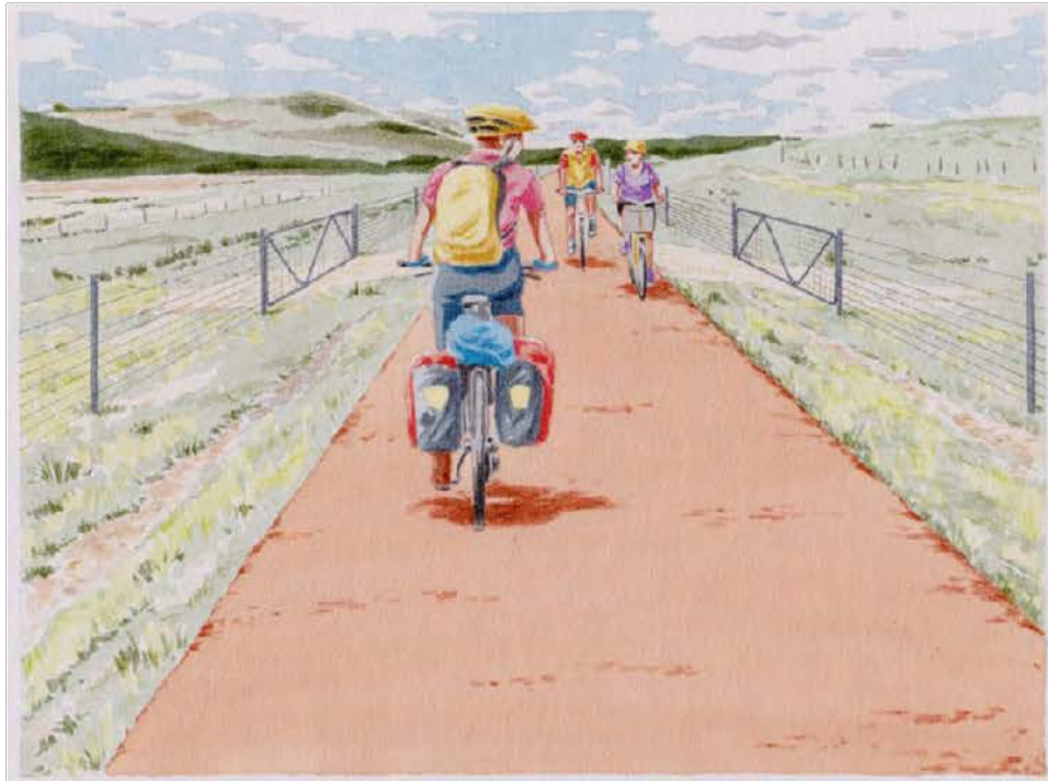
There are several options for moving stock across a rail trail. Above: crossings that are gated either side of the corridor allow the controlled passage of stock and/or machinery at certain times. Below: crossings where gates are across the rail trail, where trail users need to open/close the gate.
