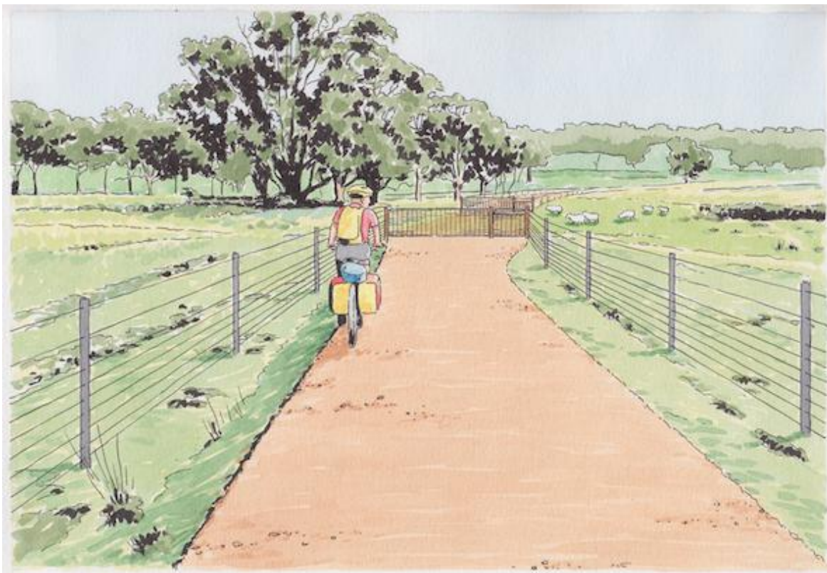
There are several options for moving stock across a rail trail. Above: crossings that are gated either side of the corridor allow the controlled passage of stock and/or machinery at certain times. Below: crossings where gates are across the rail trail, where trail users need to open/close the gate.
